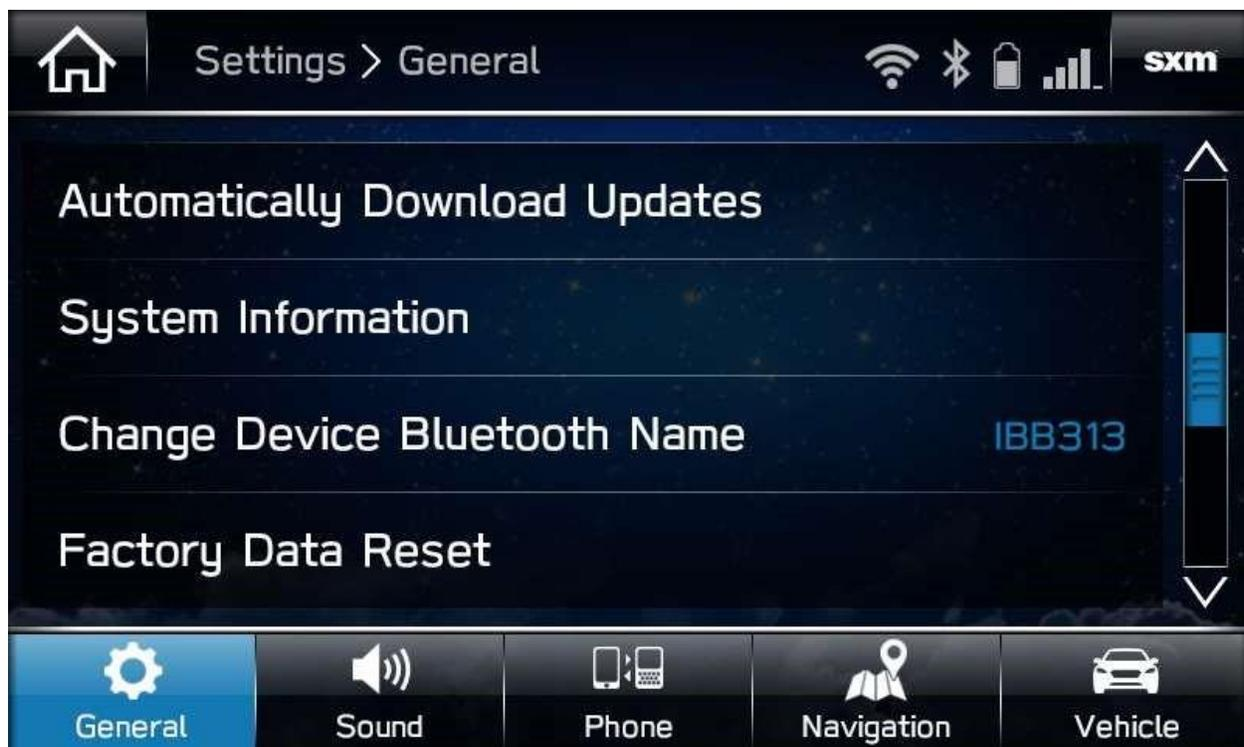
4. The current software version will be displayed. The latest version as of September 2018 is UO.18.22.20 for non-navigation units and UO.18.30.20 for navigation equipped units.
